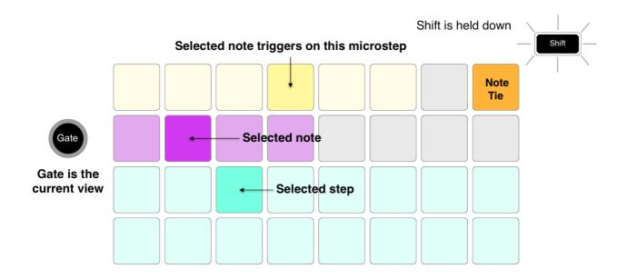
With a note selected, use the top row of pads to choose the microstep on which the note will trigger. The microstep that the note triggers on will be lit brightly, while the other microsteps will be dim. Each note may trigger only once per microstep.
